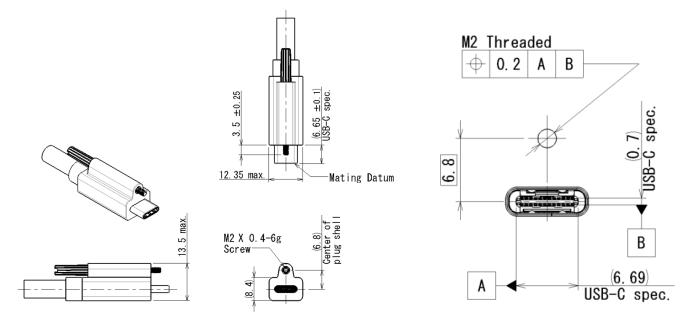
The USB-C hardware connector on the OLVX-IMU01-9D is designed to be compatible with the standard single screw USB Type-C locking plug revision 1.0 as elaborated by the USB-IF Device Working Group in 2016. Please find further details in the figure above and <u>here</u>.
